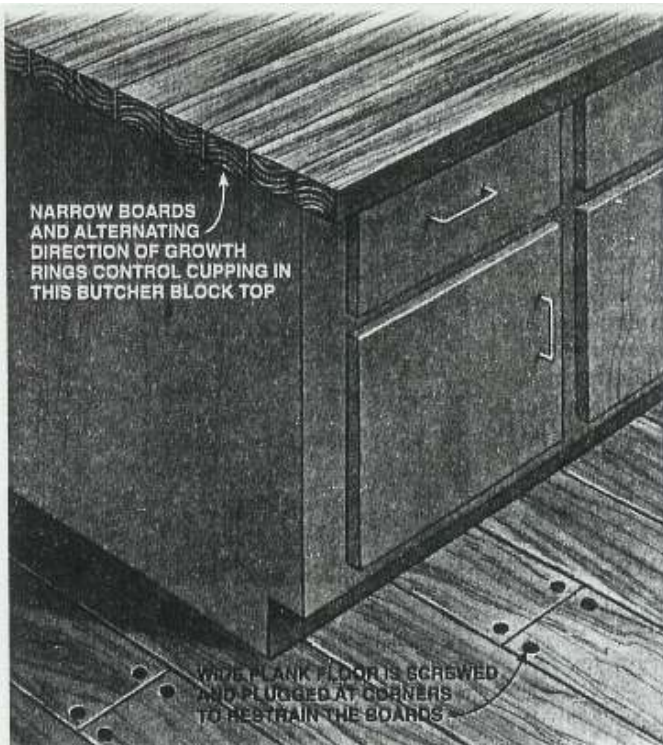
FIGURE D DESIGNS TO PREVENT CUPPING. The cupping of flat-sawn boards has to be accommodated in construction too. Many times the wood just has to be fastened down securely, but using narrower boards also helps.
